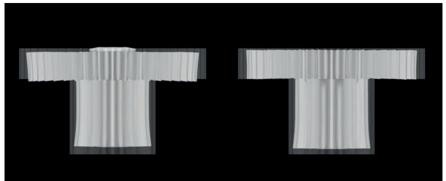
Fig. 4. Deformation of the customer model versus that of the optimized geometry, with 5:1 scaling. The greatest improvement was obtained with the model having the most ribs © MS-Schramberg
